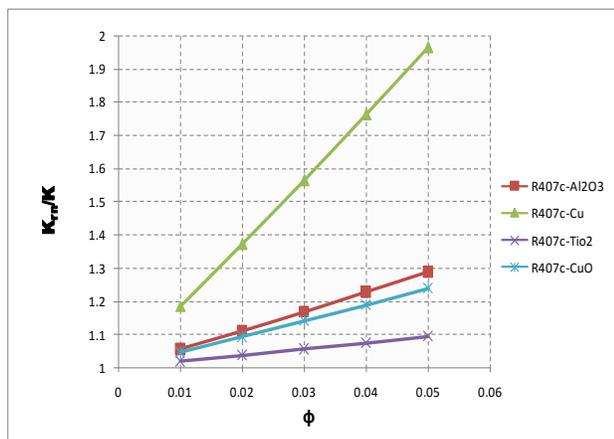
Fig.17. Variation of Thermal conductivity Ratio with volume fraction ( $\phi$ ) of R407c using different nanoparticles
