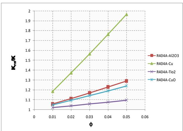
Fig.19. Variation of Thermal conductivity Ratio with volume fraction ( $\phi$ ) of R404A using different nanoparticles
