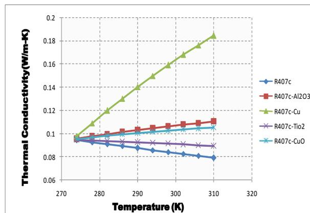
Fig.3. Variation of Thermal conductivity with Temperature of R407c using different nanoparticles
