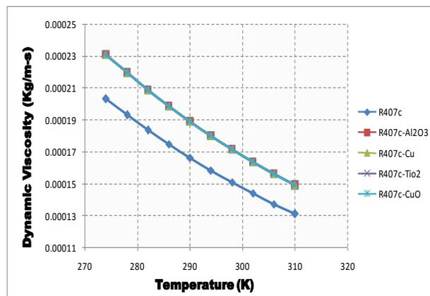
Fig.9. Variation of Dynamic viscosity with Temperature of R407c using different nanoparticles
