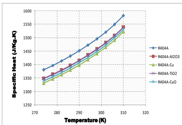
Fig.13. Variation of Specific heat with Temperature of R404A using different nanoparticles
