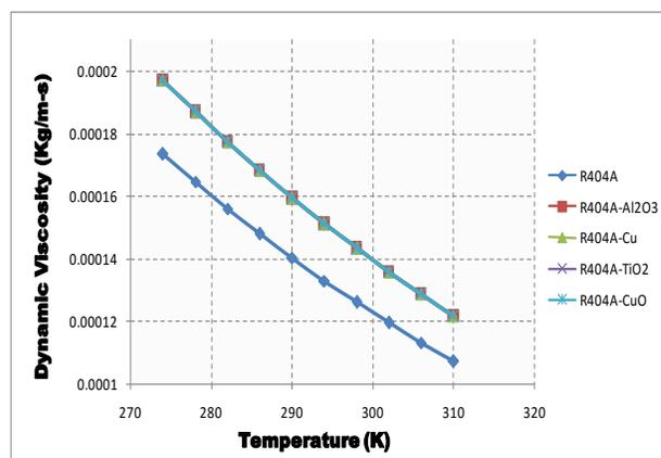
Fig.10. Variation of Dynamic viscosity with Temperature of R404A using different nanoparticles
