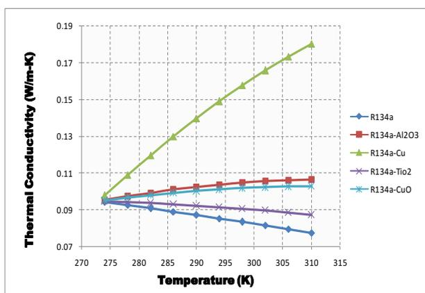
Fig.2. Variation of Thermal conductivity with Temperature of R134a using different nanoparticles
