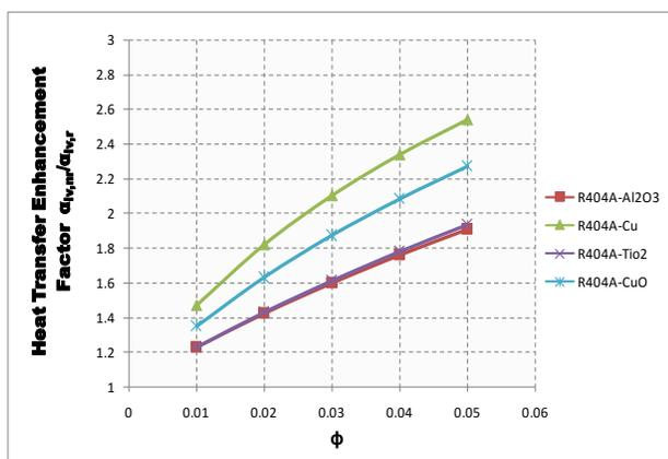
Fig.28. Variation of Heat transfer Enhancement Factor with volume fraction ( $\phi$ ) of R404A using different nanoparticles
