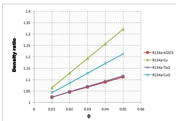
Fig.15. Variation of Density Ratio with volume fraction ( $\phi$ ) of R134a using different nanoparticles
