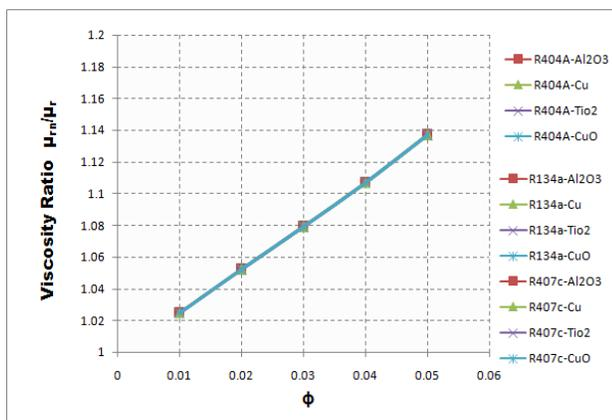
Fig.23. Variation of Viscosity ratio with volume fraction ( $\phi$ ) of all Nano refrigerant
