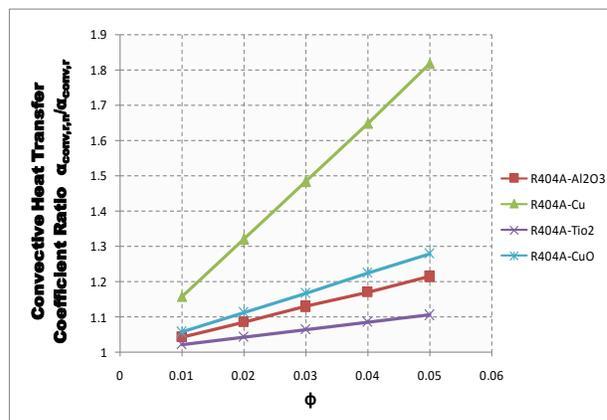
Fig.25. Variation of Convective heat transfer coefficient ratio with volume fraction ( $\phi$ ) of R404A using different nanoparticles
