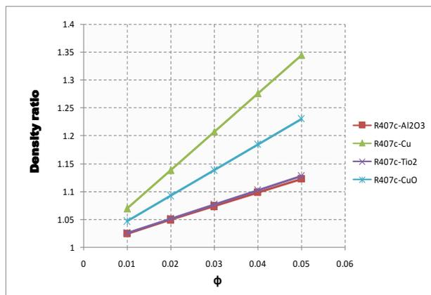
Fig.14. Variation of Density Ratio with volume fraction ( $\phi$ ) of R407c using different nanoparticles
