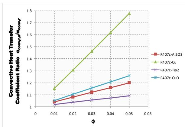
Fig.24. Variation of Convective heat transfer coefficient ratio with volume fraction ( $\phi$ ) of R407c using different nanoparticles
