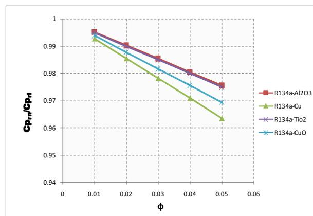
Fig.22. Variation of Specific heat ratio with volume fraction ( $\phi$ ) of R134a using different nanoparticles
