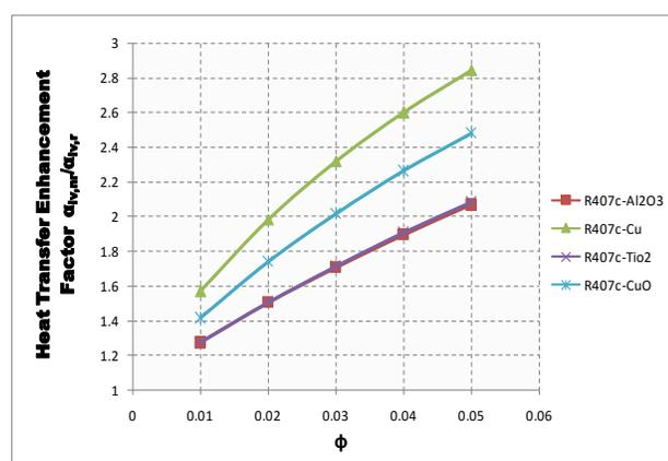
Fig.29. Variation of Heat transfer Enhancement Factor with volume fraction ( $\phi$ ) of R407c using different nanoparticles
