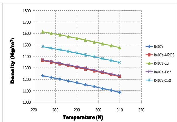
Fig.7. Variation of Density with Temperature of R407c using different nanoparticles
