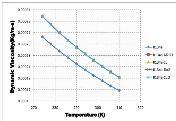
Fig.8. Variation of Dynamic viscosity with Temperature of R134a using different nanoparticles
