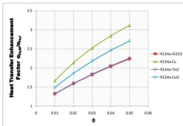
Fig.27. Variation of Heat transfer Enhancement Factor with volume fraction ( $\phi$ ) of R134a using different nanoparticles
