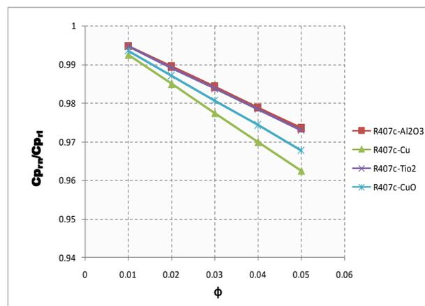
Fig.20. Variation of Specific heat ratio with volume fraction ( $\phi$ ) of R407c using different nanoparticles
