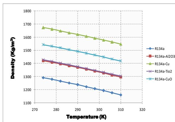
Fig.5. Variation of Density with Temperature of R134a using different nanoparticles
