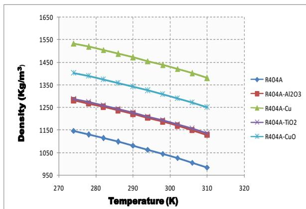
Fig.6. Variation of Density with Temperature of R404A using different nanoparticles
