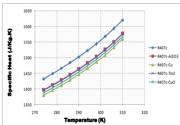
Fig.11. Variation of Specific heat with Temperature of R407c using different nanoparticles
