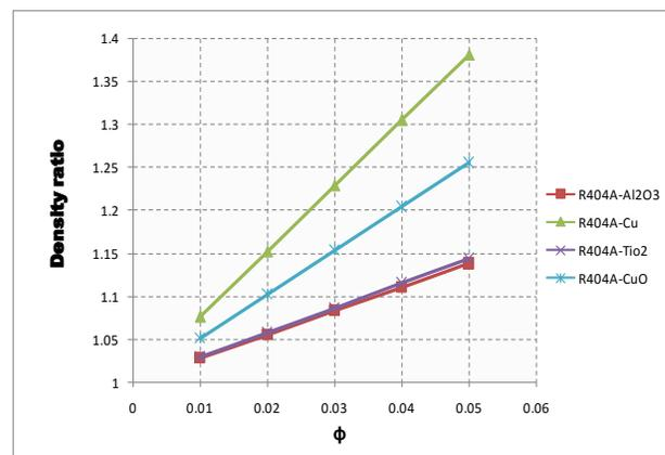
Fig.16. Variation of Density Ratio with volume fraction ( $\phi$ ) of R404A using different nanoparticles
