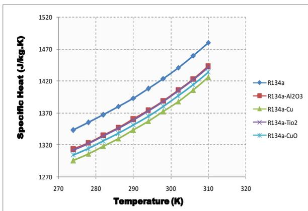
Fig.12. Variation of Specific heat with Temperature of R134a using different nanoparticles
