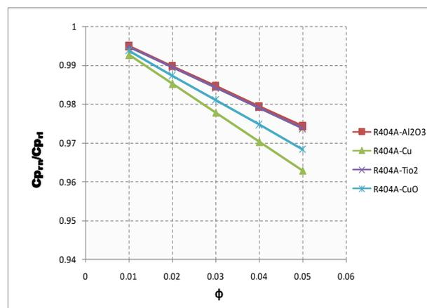
Fig.21. Variation of Specific heat ratio with volume fraction ( $\phi$ ) of R404A using different nanoparticles
