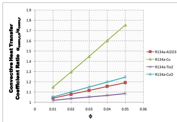
Fig.26. Variation of Convective heat transfer coefficient ratio with volume fraction ( $\phi$ ) of R134a using different nanoparticles
