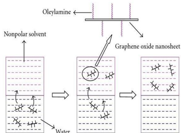
Figure 1: Schematic illustration of the phase transfer process
