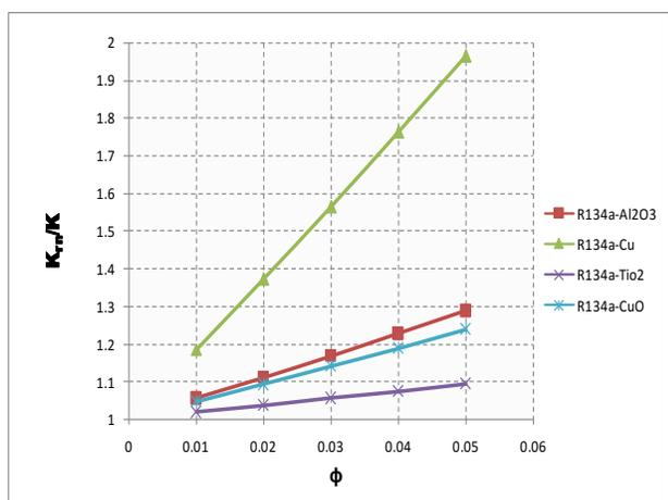
Fig.18. Variation of Thermal conductivity Ratio with volume fraction ( $\phi$ ) of R134a using different nanoparticles
